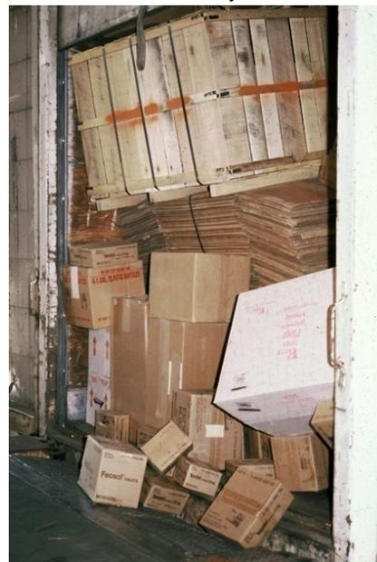
When cargo is in a closed van the chance of losing the load is minimal, but the damage to cargo and to the stability of the vehicle is at risk. This picture has a heavy item up high and no bracing or load locks to prevent the load from shifting. This can drastically impact the center of gravity and produce adverse weight distribution that will disrupt the safe operation of the vehicle. Not only that, but would you like to unload this!!!
