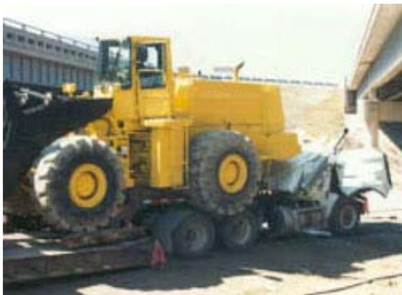
**Myth 2** – Load securement is not necessary except when on a highway.
